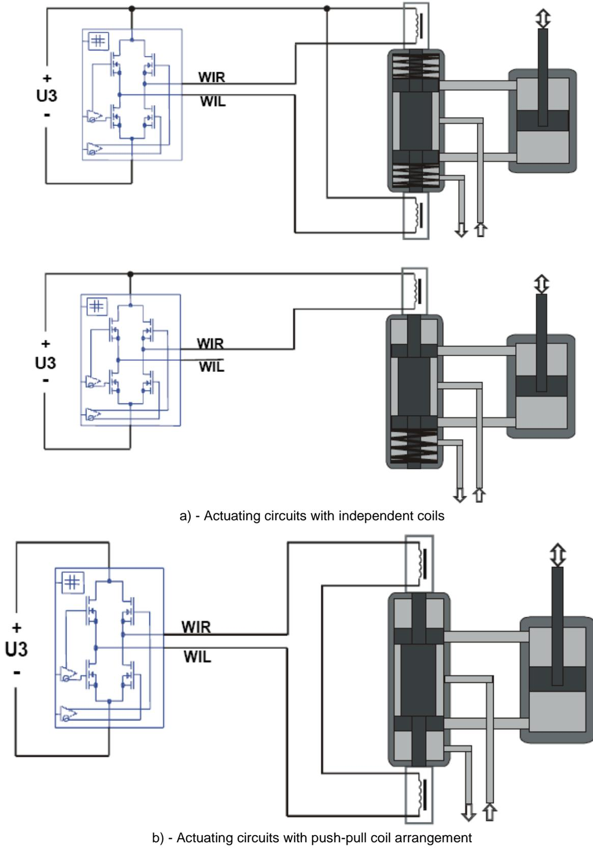
a) - Actuating circuits with independent coils
