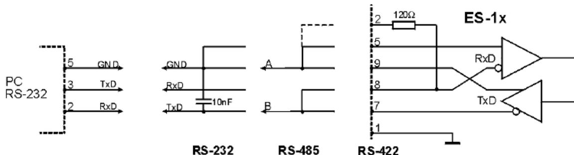
Fig. 1 COM1 and COM 2 (RES422/RS485/RS4232) serial channels of the controller
