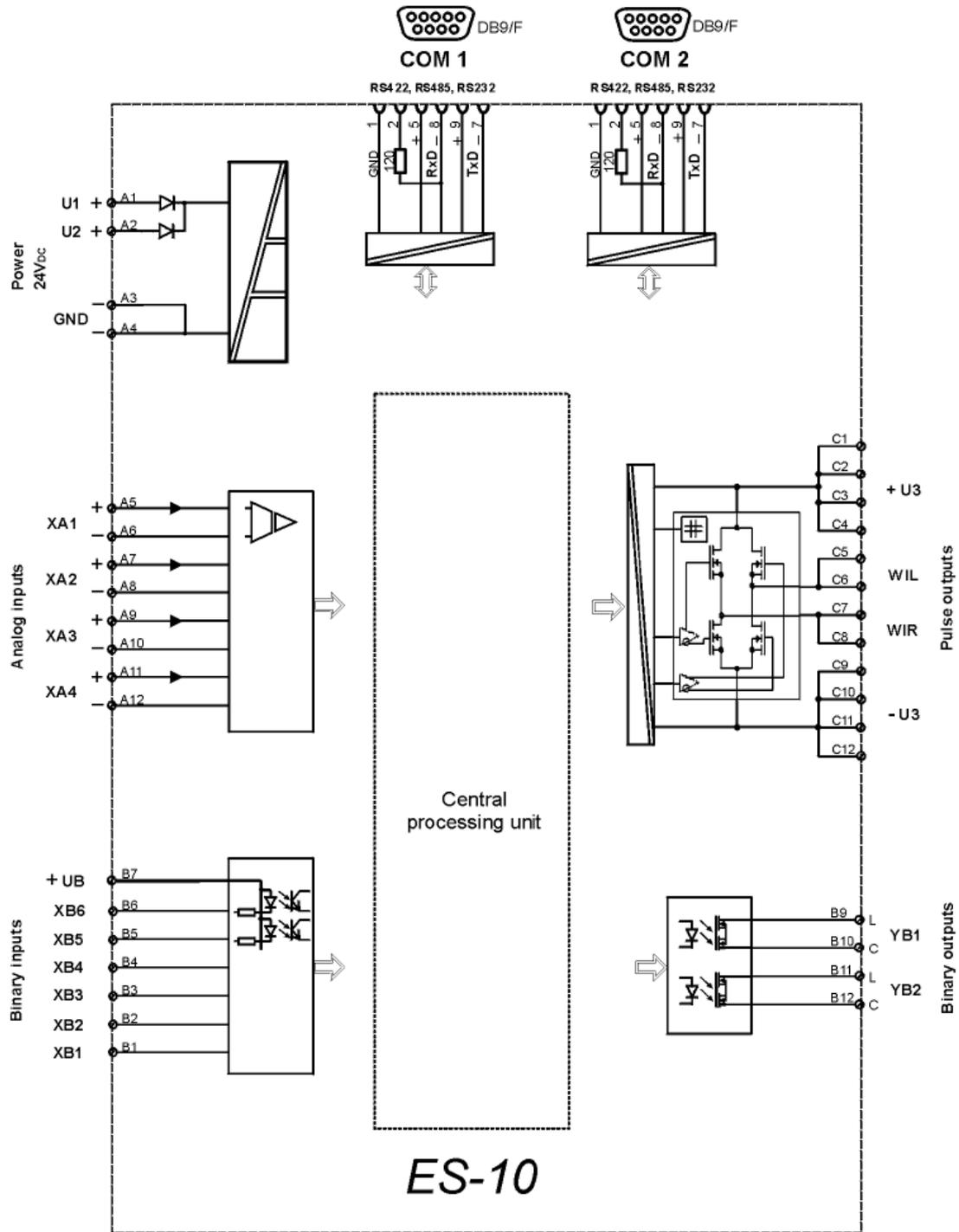
Fig.2. Block diagram of the controller
